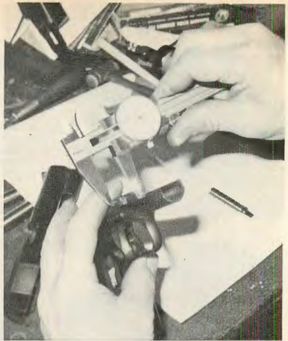
Above: Rails on frame are then reshaped, and redesigned to fit within .002 the grooves in slide. Here Starks checks rail measurements during handfitting process.
